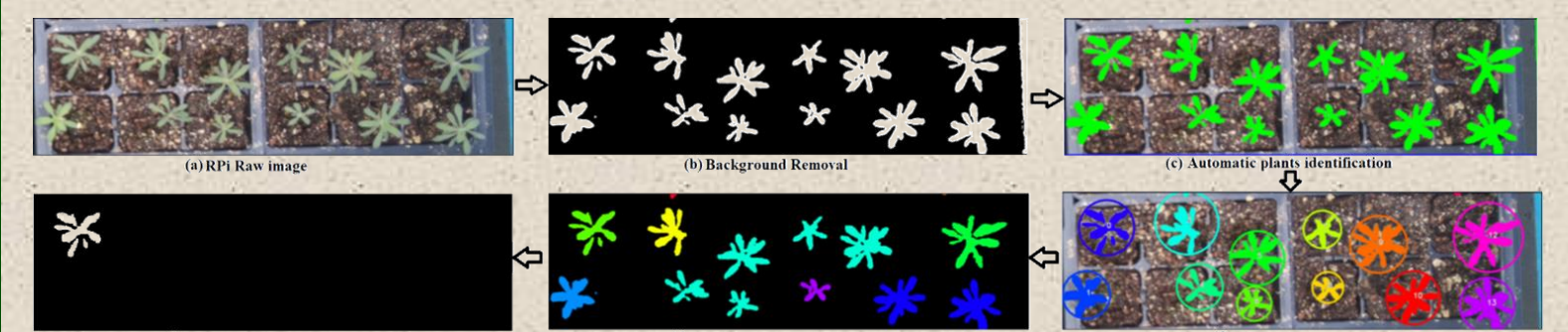
Fig. 9 RPI image processing and analysis workflow, (a) RPI raw image, (b) Background removal, (c) Automatic plants identification, (d) Plant clustering, (e) Individual plant extraction, (f) Extracted single plant
